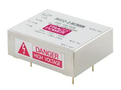
The PHV series are regulated miniature high voltage power modules using SMD and hybrid technology. They are designed for PCB mounting. The use of high stability components guarantees a minimal temperature drift and a very stable output voltage. Typical applications for these HV power supplies are photomultiplier tubes, gas chromatography, analytical instruments and wherever where small size and high output voltage stability is requested.
