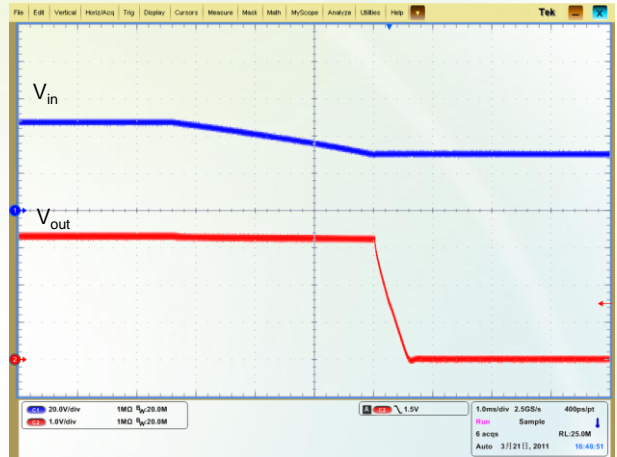
Figure 12: Shutdown by power off
